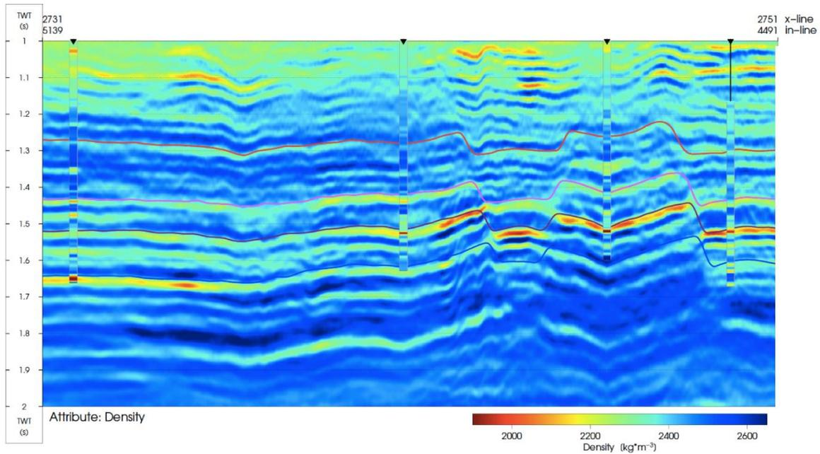
Figure 1. Absolute density inversion results – (top) PP (bottom) PP-PS. Note the improved resolution in the PP-PS events for example in the central graben structure and across the E8 horizon. Four well traces are inserted for comparison purpose.
